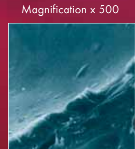
Cross linked and chemically expanded LDPE foam
